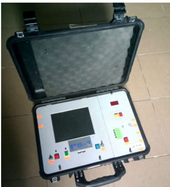
The prototype of the device for quick detection of unexploded ordnance and mines.jpg
